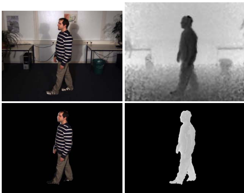
Fig. 4. Depth keying: Original color and depth image. Bottom: depth-based segmentation.
