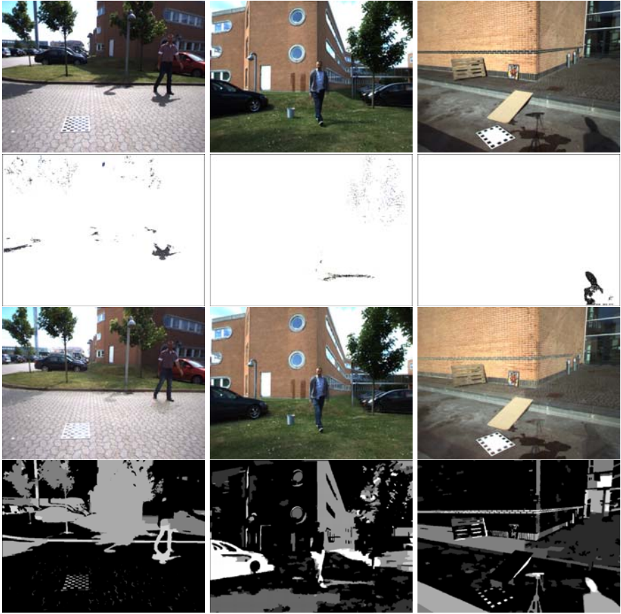
Fig. 10. First row: original images from three different sequences. Second row: shadows detected by approach described in this paper. Third row: shadows removed with graph cuts based approach. Fourth row: level of shadow (brighter areas represent a deeper shadow level).
