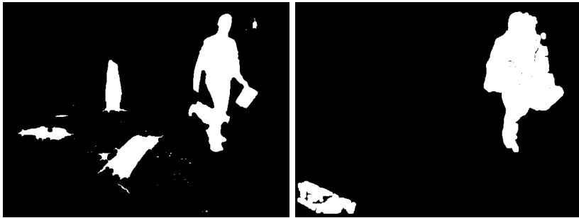
Fig. 3. Left: Pixels (frame 137) determined by the Codebook method as being different from the trained color background model. Right: Pixels (also frame 137) determined as being different from the disparity background model.
