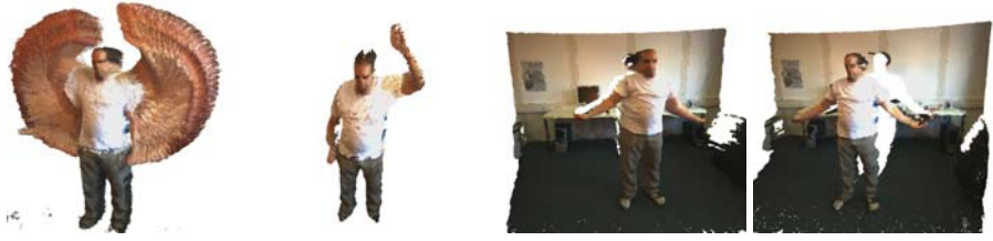
Fig. 7. Space-Time Video: All elements in the octree (left), selected time instance of the animation sequence (second), rendered views with background (right).
