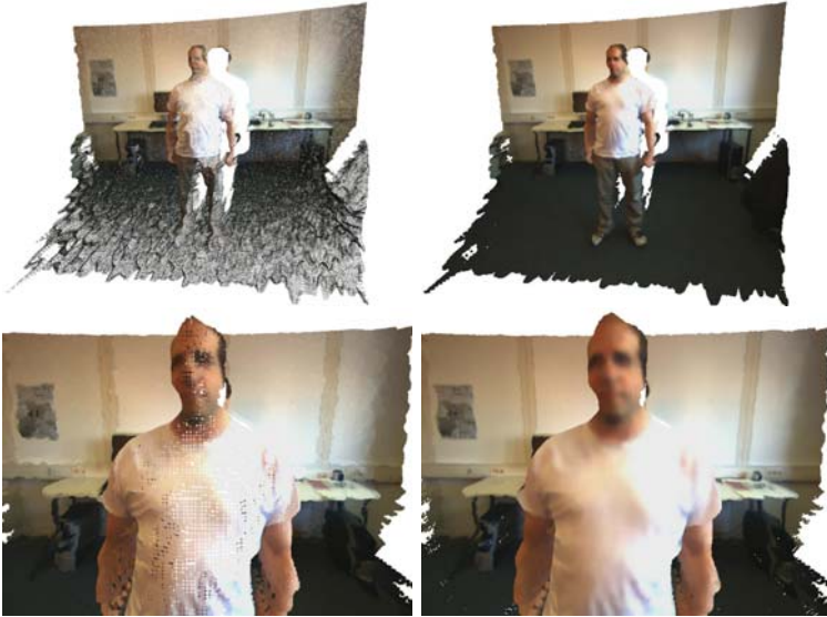
Fig. 2. Comparison of point rendering (left) and point splatting (right)
